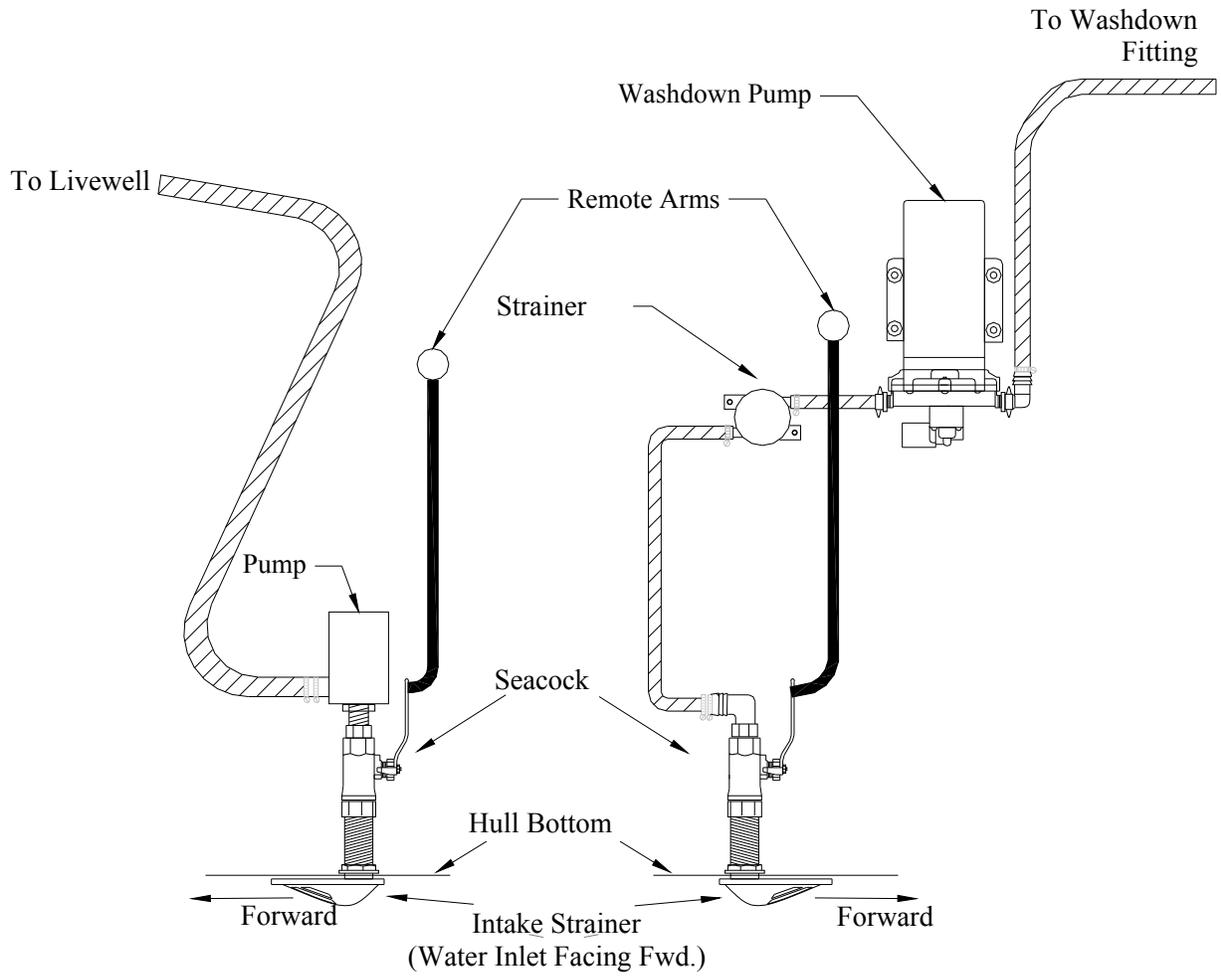
***Thru Hull Detail***
